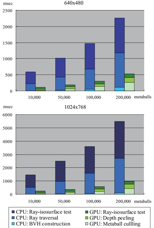
**Figure 8:** Graphs of the computational times for the CPU and GPU versions when rendering the scene in Figure 1.
