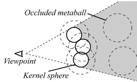
**Figure 7:** Culling metaballs using kernel spheres. The metaballs in the gray region are hidden by kernel spheres.
