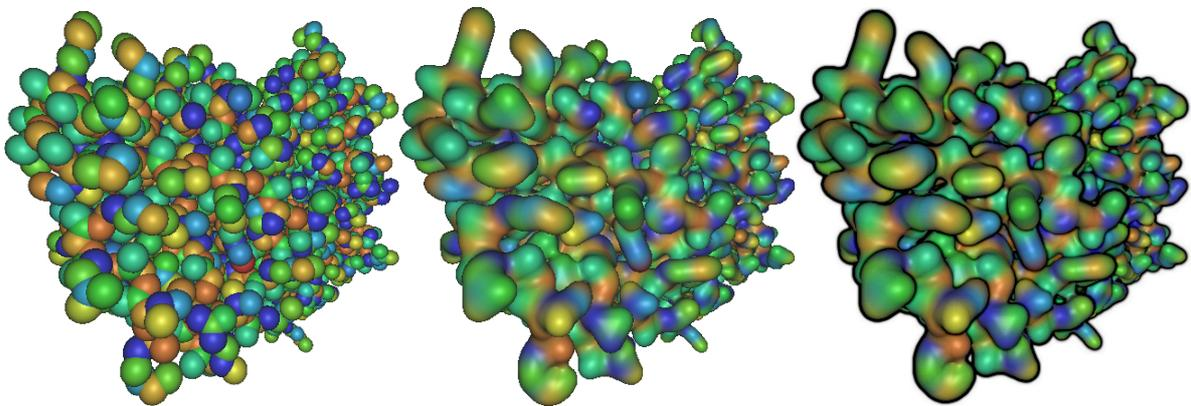
**Figure 11:** Visualization of a molecular dynamics simulation with 2,878 metaballs. When simply drawing a sphere for each atom (left, 3971.9 fps), the bonds between the atoms are hard to see. When using our method they become more clear (center, 22.9 fps). Applying Luft et al.'s image enhancement method [LCD06] increases the feeling of depth perception (right, 22.8 fps).
