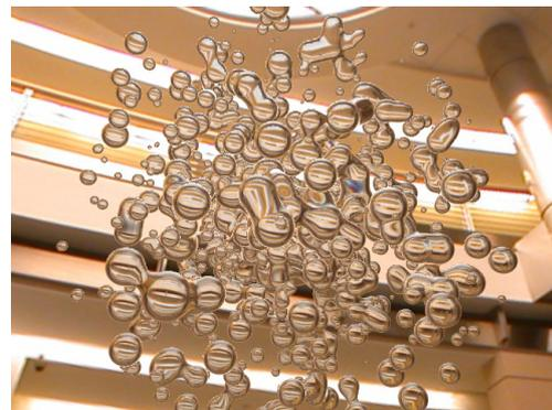
**Figure 1:** Screenshot from an animation with 1,000 moving metaballs, rendered in 640×480 at 23.1 fps. Unlike polygonization, even small particles are rendered smoothly.
