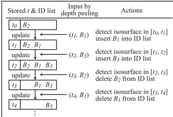
**Figure 5:** Updating the list of metaball IDs for the viewing ray  $R_1$  in Figure 2.
