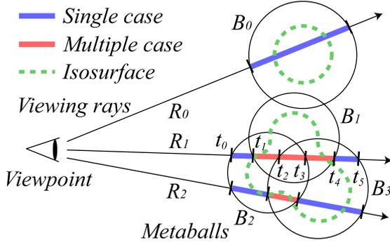
**Figure 2:** The basic framework for rendering metaballs.  $\{B_0, \dots, B_3\}$  are the metaballs' IDs, and  $\{t_0, \dots, t_5\}$  the parameters for each intersection point along the ray  $R_1$ .
